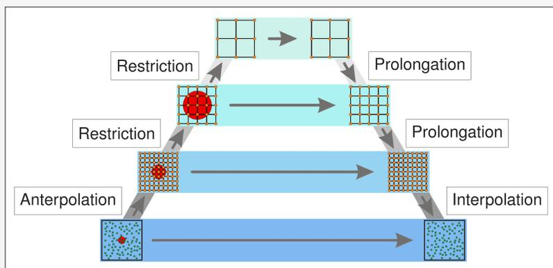
Schematic representation of one step of the Multilevel Summation algorithm with 3 grid levels
