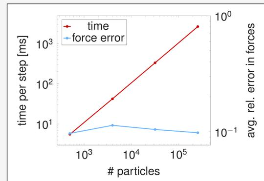
Total timings per step and error in forces for 500, 4000, 32000 and 256,000 particles.
